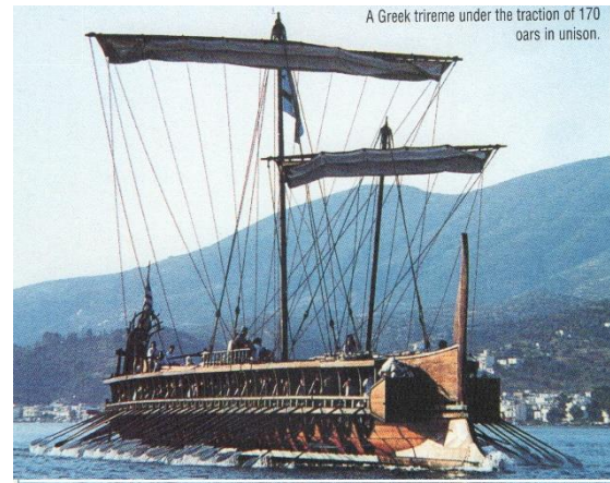
A replica of an ancient Greek trireme in which 170 Athenians rowed in 3 tiers in unison
